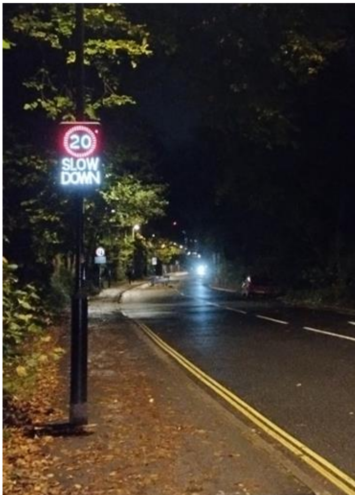
Vehicle Activated Signage example (Woolston)
