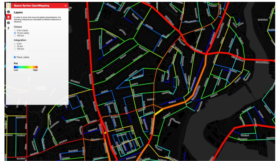
Map 5. Choice model of Portswood movement infrastructure – vehicular movement – 10km rank (Source Space Syntax)
